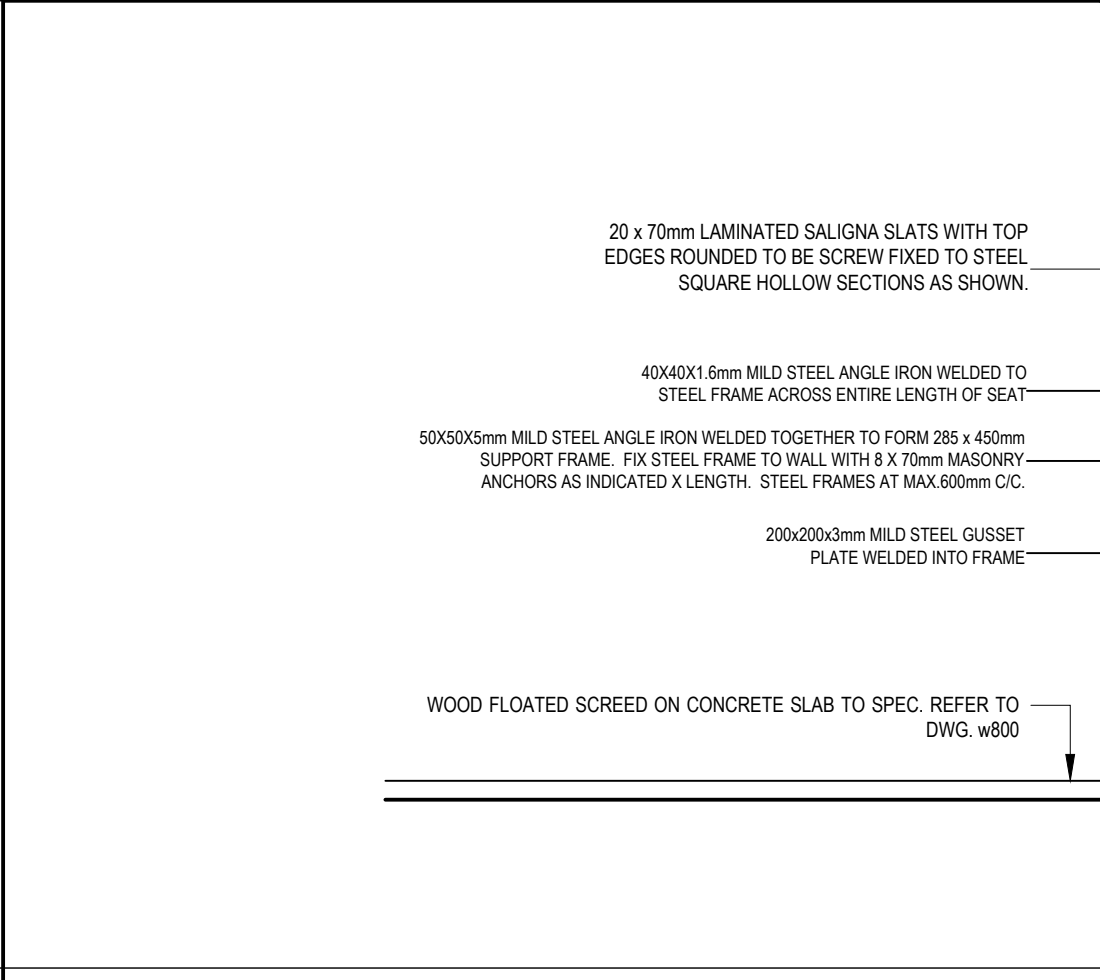
DETAIL 33.3: SECTIONAL ELEVATION A SCALE 1:20
